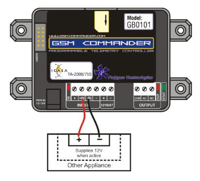
Please keep in mind that these inputs are designed for 5V to 12V operation.
