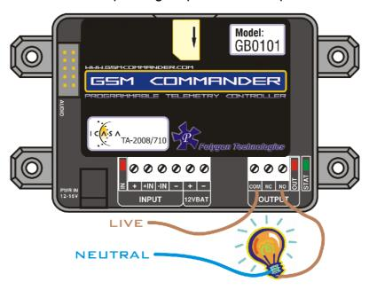
The output can be used to control devices and appliances, and is rated for 8A DC. It may be used to control most types of electrical loads, excluding AC motors above 500W.
