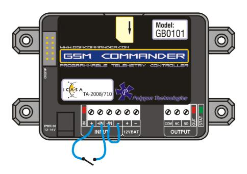
You may need an input to activate when power is supplied from some other unit. A good example will be a burglar alarm that applies power to the wires going to the siren. In such a case, it will be a simple matter of connecting the positive wire to the IN+ input, and the negative wire to the IN- input.
